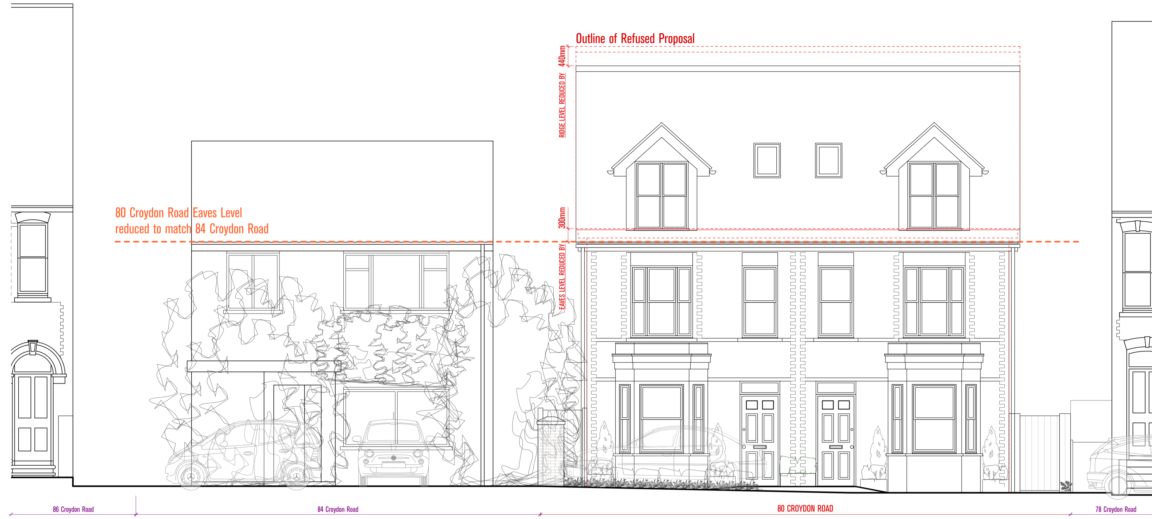
80 Croydon Road Street Scene (Elevation A-A)
